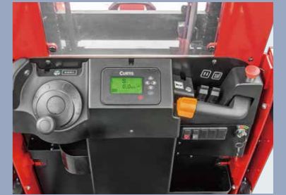
The FREE accelerator lever with sensor switch, as standard configuration, can prevent mis-operation during the work
